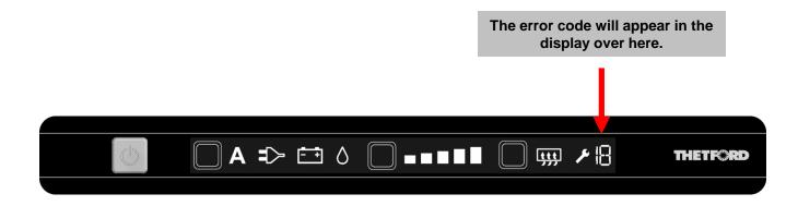
!!! Note: When supply voltage 12 VDC (low current voltage) is not available, no error code will be given. When 12 VDC is available the green power LED will be on !!!
