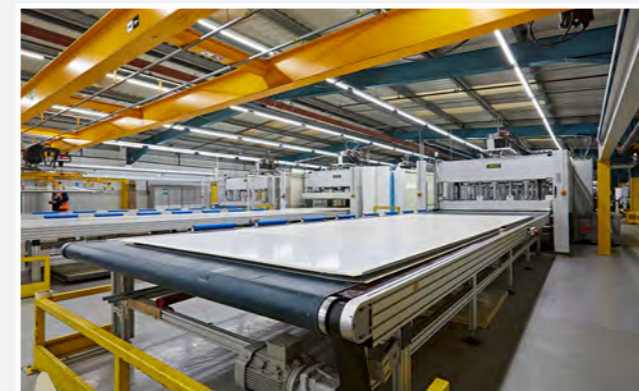
'SMART' GRP sidewall during the production process.
